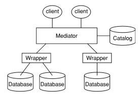
Fig. 12. Wrapper architecture of heterogeneous databases.
