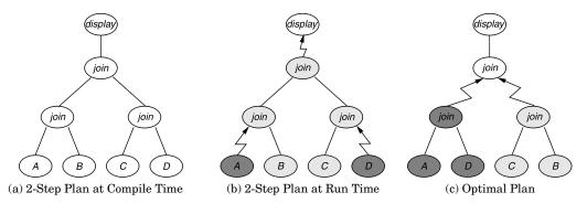
Fig. 11. Increased communication cost due to two-step optimization.
