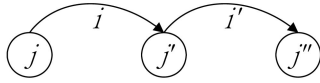
Fig. 1. Shift the task i to agent j' and i' to agent j'' simultaneously.
