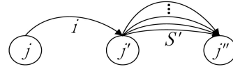
Fig. 2. Shift a VS i to node j' and S' to node j'' simultaneously.
